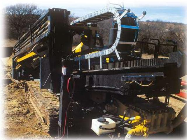
**Rack-and-pinion drive.** This simple system provides smooth operation. The D100x120 Series II unique narrow rack-and-pinion design helps maintain a small footprint for access into congested areas. The rack is sectionalized and bolts on for easy repair or replacement.
