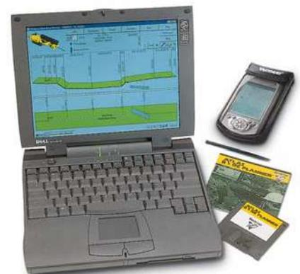
**The efficient, economical way to plan a bore.** Vermeer ATLAS BORE PLANNER® software heightens professionalism by aiding the operator in preplanning the bore and comparing the planned bore path with the actual bore path. The Vermeer FieldCalc™ system combines software and a hand-held computer to provide job site calculations, including setback distance, pullback time, and point-to-point calculations.
