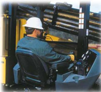
**The state-of-the-art operator's station** is elevated with an electrically operated swivel and tilt control seat. Dual joysticks control functions for mudflow, breakout vise, and throttle and are integrated into the thrust and rotation controls. This feature provides the operator fingertip control over repetitive drill functions. Drilling pressure gauges are located within operator line of sight.
