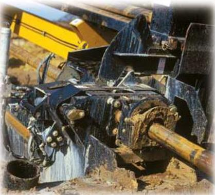
**The floating vise feature** allows the breakout system to clamp the full rod upsets during breakout of the lower and upper joints. The D100x120 Series II uses replaceable breakout dies and does not require backup wrenches.
