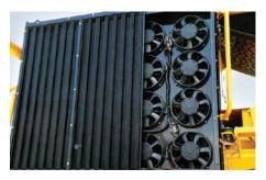
COOLING SYSTEM. To reduce sound levels and maximize power to material processing functions, the cooling system includes electrically powered, variable speed reversible fans.
