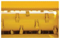
**DUPLEX DRUM.** To reduce daily maintenance time, the patented Series II duplex drum, designed with reversible tips and hammers, is available.
