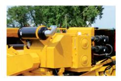
ENGINE. Fully enclosed IVECO/Fiat Power Train (FPT), 445 hp (332 kW) engine.
