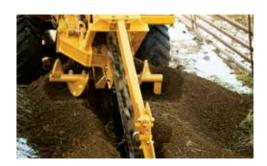
MAKE SENSE OF YOUR TRENCH. When difficult conditions are encountered while trenching causing a sudden drop in engine speed, the TrenchSense<sup>™</sup> feature automatically pauses the forward motion of the tractor to prevent engine shutdown and recalibration of the machine controls. Once pre-set engine and trencher speed recovers, forward AutoCreep resumes. The sequence occurs within seconds and requires no operator adjustment.
