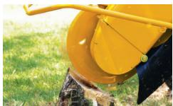
YELLOW JACKET™ CUTTER SYSTEM. The Vermeer-exclusive Yellow Jacket cutter system is designed to provide faster, easier serviceability, as well as extended pocket and tooth life.
