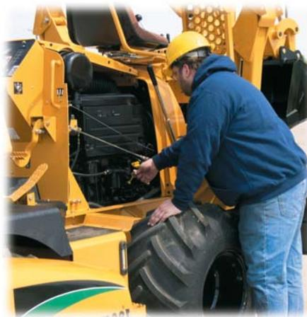
**Convenience and accessibility.** Removable shields on both sides of the machine provide easy access to the engine and place the oil dipstick, filters and fill points within easy reach.
