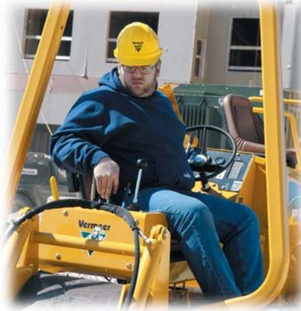
**Smooth operation.** For added comfort, the operator's station rotates 90 degrees allowing the operator to select five different positions. The attachment controls rotate with the operator providing easy and consistent reach at all times.
