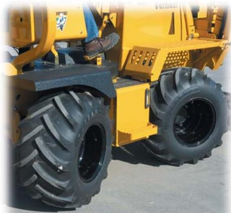
**Freedom to move.** The RT650's tight turning radius, with steerable rear planetary axle, provides excellent maneuverability in confined work areas.
