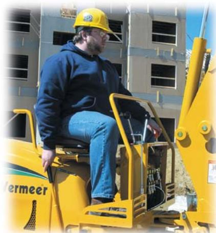
**Control at your fingertips.** Standard backhoe remote controls for the start, creep, idle and stop functions permit the operator to reposition the machine without leaving the backhoe operator's station.
