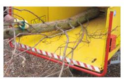
BOTTOM/SIDE FEED STOP BARS. The bottom/side feed stop bar system is strategically located to make it possible for an operator to strike the bar and stop the feed, either intentionally or automatically in an emergency situation.
