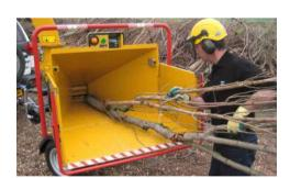
HIGH-CAPACITY INFEED. The BC160xL has a 16 cm x 20 cm (6.3" x 7.9") infeed opening to help boost productivity by reducing the need to trim material before feeding into the chipper.
