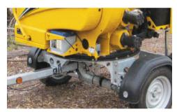
360° ROTATING TURNTABLE. Allows the chipper infeed to be rotated to face where the material is located for ease of feeding and greatly increases safety when working along the roadside by keeping the operator away from road traffic.
